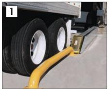
As the vehicle approaches the loading dock, it is guided into position between the wheel guides.
