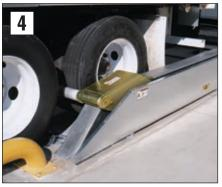
The locking arm automatically sizes the tyre and rises to its full height against the tyre.
